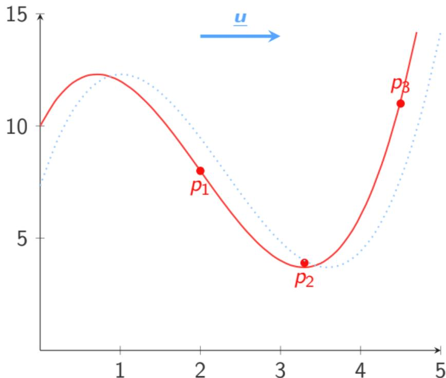
$$- \quad \underline{u} \quad \frac{\partial C}{\partial x} = \frac{\partial C}{\partial t}$$
